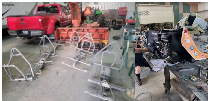
The Trike frame had to be extend by 6" for the new motor to fit.
