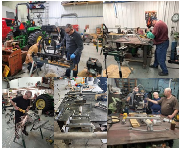
The Trike frame had to be extend by 6" for the new motor to fit.
